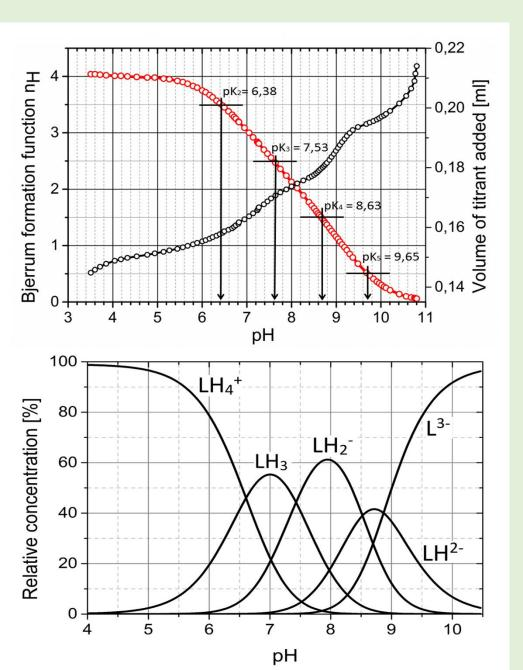
The pH-potentiometric titration curve of acidified Eltrombopag plus HCl titrated with KOH is plotted with the Bjerrum protonation function indicating pK values.
