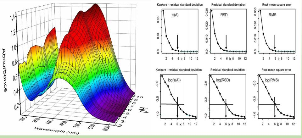
The 3D-absorbance-response-surface concerning 71 measured absorption spectra of protonation equilibria for 9,5 .  $10^{-5}$  M Eltrombopag in dependence on pH at 25°C. The Cattel's scree plot of the Wernimont-Kankare procedure for the determination of the rank of the absorbance matrix of Eltrombopag  $k^* = 6$  leads to six light-absorbing species in the mixture,  $n_c = 6$ , with the use of Kankare's s(A), RSD and RSM.
