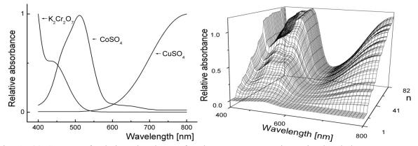
Fig. 1: (a) Spectra of relative absorbance for three components in a simulated three-components system in mixture, potassium bichromate - cobalt(II) sulphate - copper(II) sulphate, with r = 3, n = 82, m = 41 and SER = 1570, S-Plus, (b) 3D-relative absorption spectra forms the input of INDICES.
